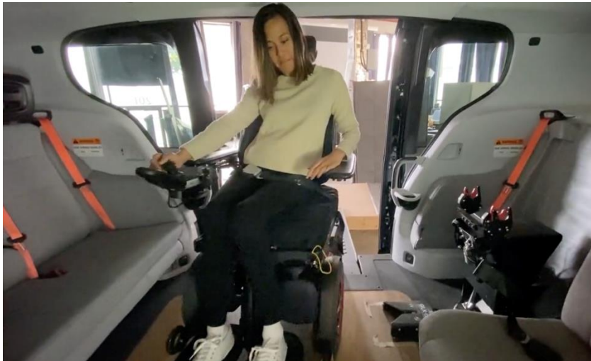
Figure 5-C: Wheelchair integration concept in a Cruise Origin
