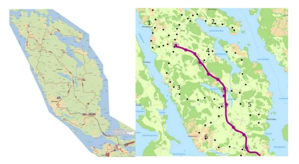
The idea is to replace the above bus line network (left above) with the following (right above): a trunk line (purple line) as well as stops for boarding (purple dots) and transfers from/to DRT to trunk line (purple dots with a pentagon around them). The black dots symbolize former bus stops that we assume will be used for boarding and disembarking for the DRT traffic.
