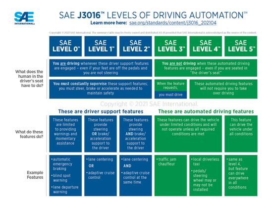
The SAE (Society of Automotive Engineers) J3016 Levels of Driving Automation is the official definition of autonomy level. | Image credit: SAE International.
