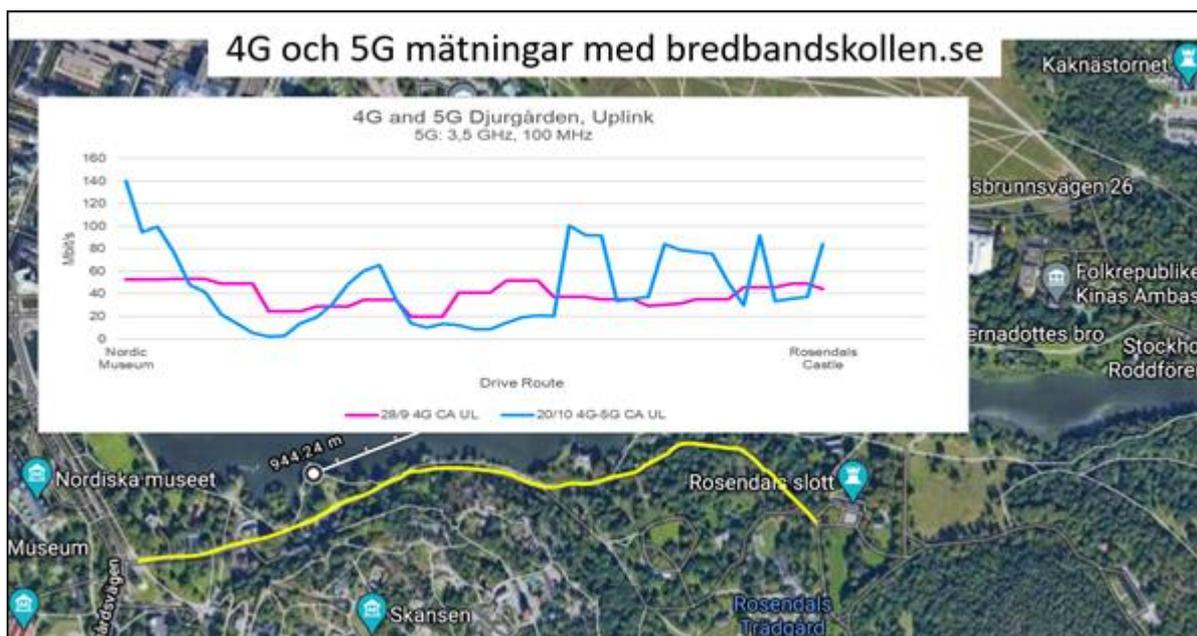
Secondly, the public 4G network consists of aggregated frequencies between 800 - 2600 MHz. 4G had a smoother and more stable level on the uplink than 5G, the 4G uplink was in some cases better than the 5G test network and in other cases worse than the 5G test network.
