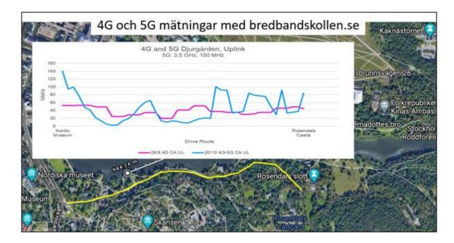
Secondly, the public 4G network consists of aggregated frequencies between 800 - 2600 MHz. 4G had a smoother and more stable level on the uplink than 5G, the 4G uplink was in some cases better than the 5G test network and in other cases worse than the 5G test network.
