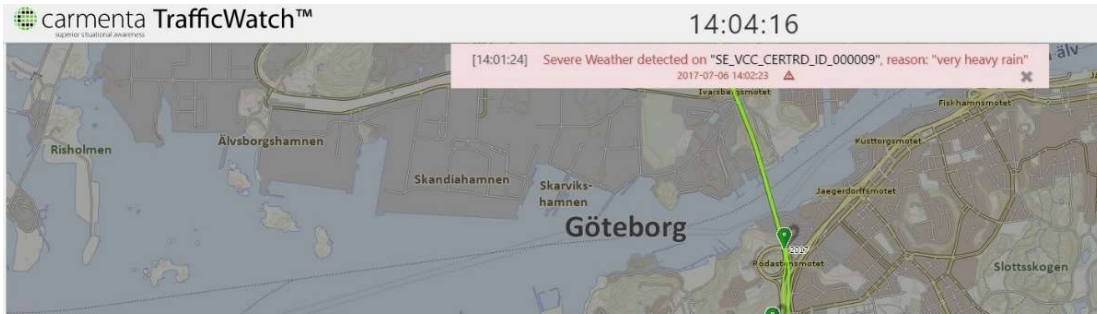
Screen dump showing the warning message that notifies the operator that a hazardous road condition has been detected on a monitored AD road segment.
